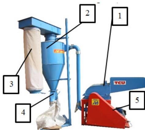
Fig. 1. **Hammer mill MC 22:** 1 – hammer mill; 2 – exhauster; 3 – cyclone with support and dust collector bag; 4 – grinding material evacuation vent; 5 – electric motor
